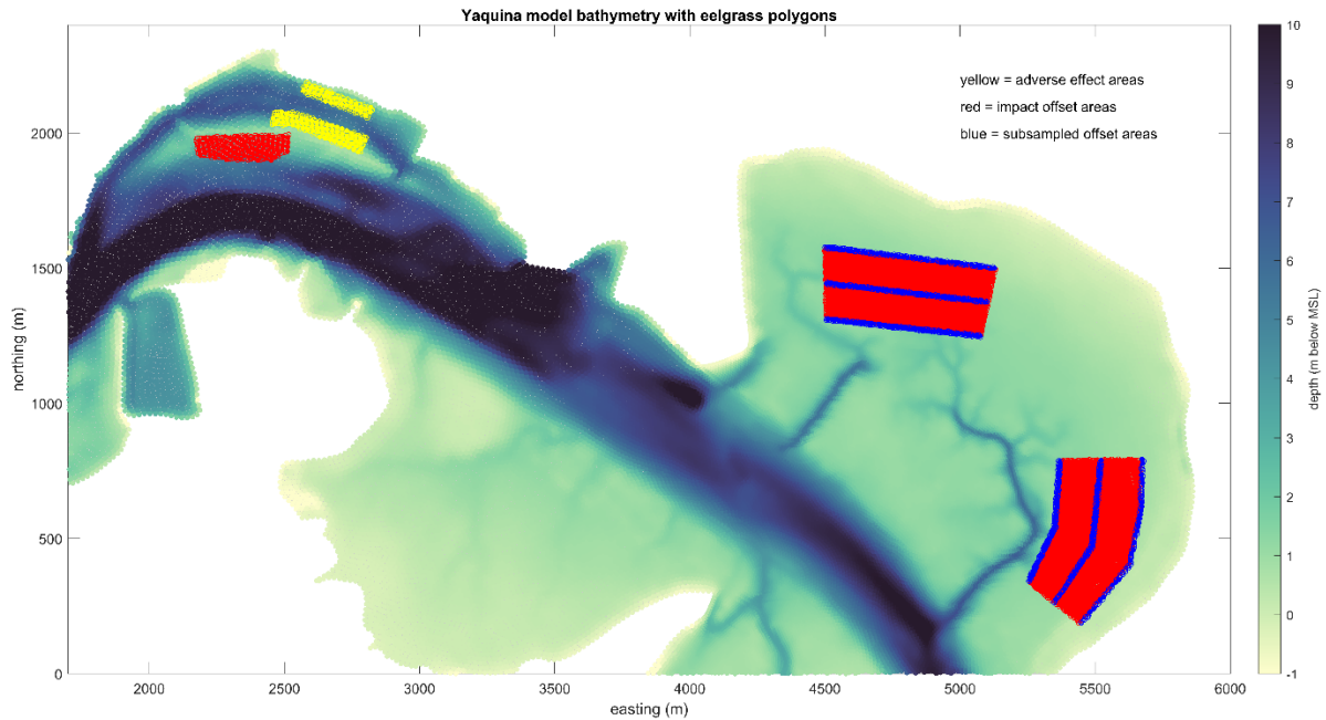
Figure 3-3. Yaquina Bay circulation model bathymetry, with polygons for areas targeted for evaluating potential eelgrass habitat suitability.
