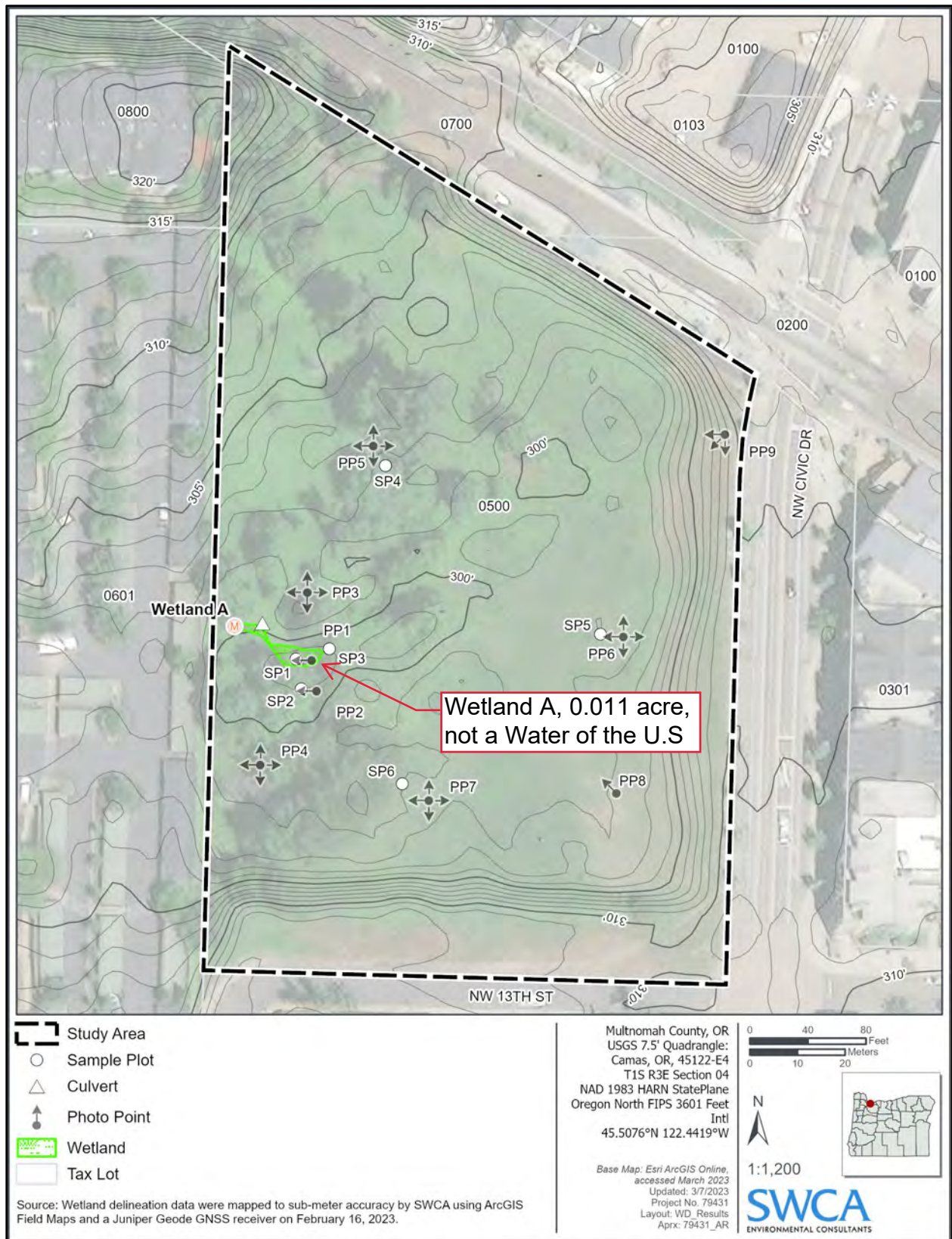
Figure 6. Delineation and photo point map with contours from LiDAR.
